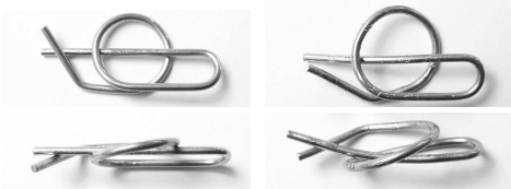
Securing pin o.k. Change the securing pin Condition of the securing pin
